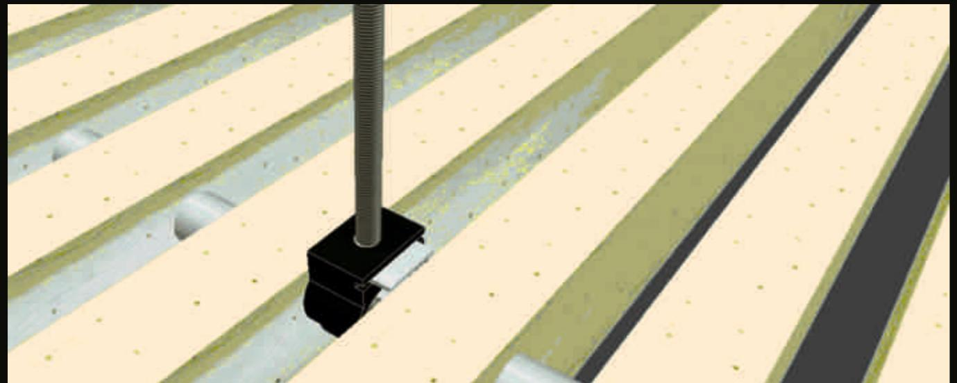
If you want the joints among the panels' heads to be more rigid, you can use plan metal elements placed in the non square edge of the panel by using the appropriate screws. This operation is not essential.
