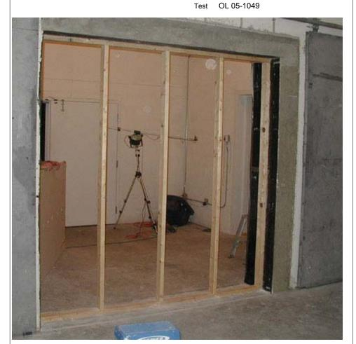
Figure 2: Wood-stud Specimen Frame in Opening
